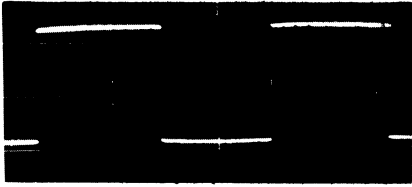
Fig. 29. Normal response to a 50 cycle square wave.
