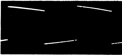
Fig. 31. Response to 50 cycle square wave when low frequency compensation is insufficient, also indicating need for L.F. adjustment.
